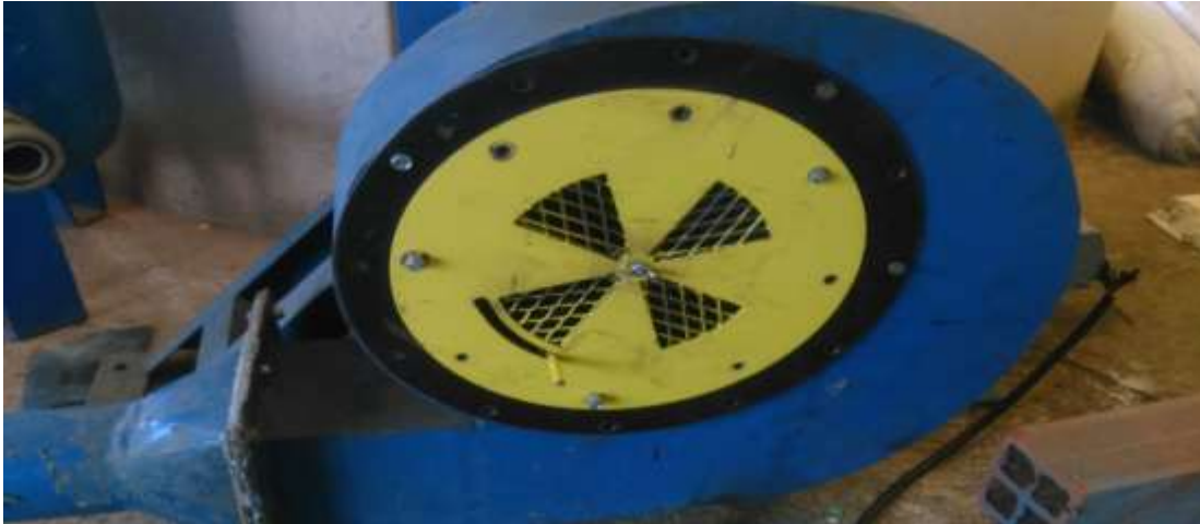
Figure 1. Diaphragm coupled to the fan for restricting the flow of air.
